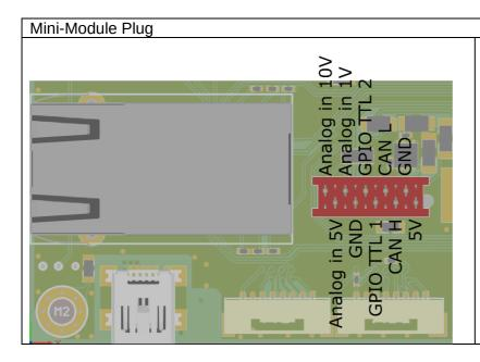
Connector: Würth Elektronik MiniModule Connector WR-MM Part Number: 690367181072
