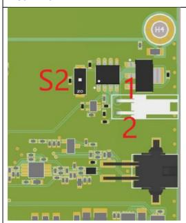
To enable the LDD apply a voltage between 3V and 30V between the Interlock + and Interlock – Pins. The Interlock Pins are galvanically isolated from the LDD.
