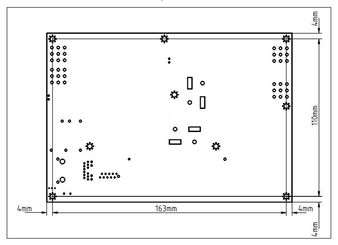
Mounting holes in the corner are 3.2 mm holes for M3 screws.
